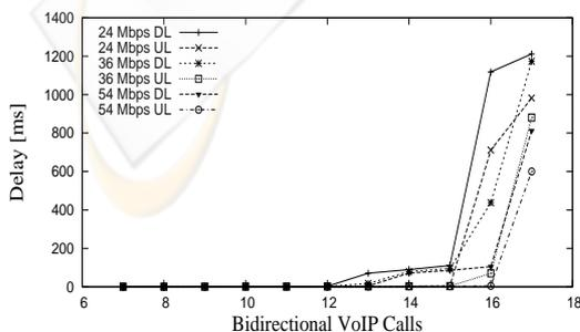
Figure 2: End-to-End Delays With Only VoIP Traffic
