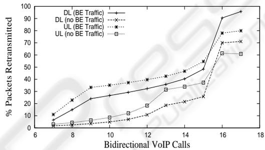
Figure 8: VoIP Packets Received After Retransmission With Best Effort Traffic at 24Mb/s
