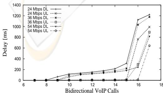
Figure 6: End-to-End Delays With Best Effort Traffic
