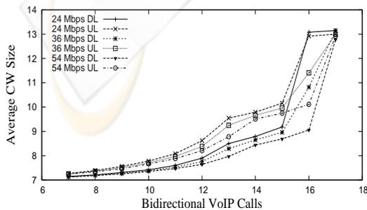
Figure 4: Contention Window Sizes With Only VoIP Traffic
