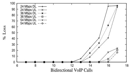
Figure 3: Loss Rates With Only VoIP Traffic
