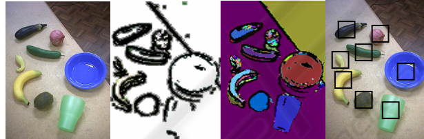
Fig. 5. Result of online scene analysis (from left to right): (a) original image frame (b) result of edge detection (c) segmentation based on the genetically tuned parameters (d) genetically tuned object classification.
