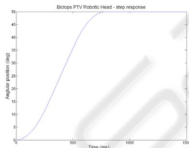
Figure 9: Biclops robotic head step response
