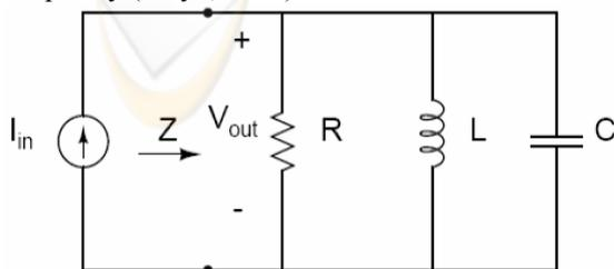
Figure 8: Parallel RLC circuit
