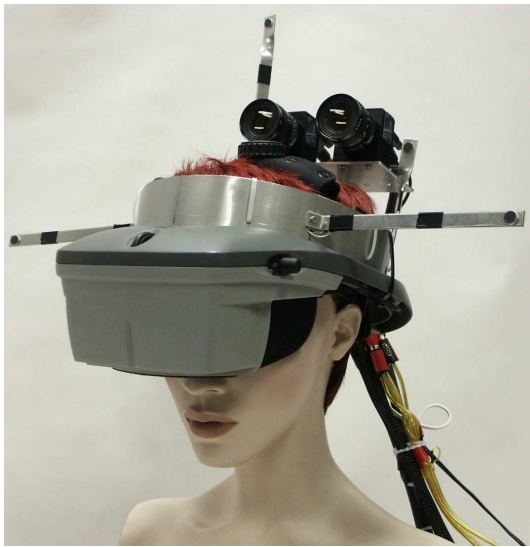
Figure 4: Experimental AR System with audio tracking.
