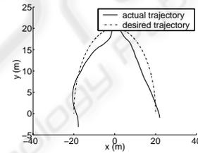
Figure 3: Evolution in the phase plane  $(x, y)$  with uncertainties without ISM
