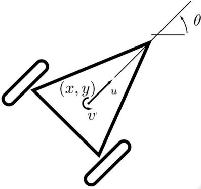
Figure 1: Unicycle robot kinematic
