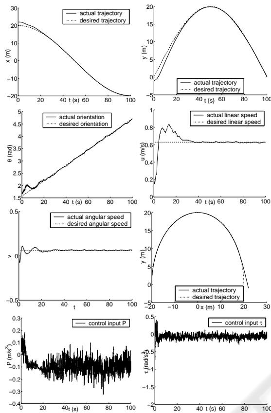
Figure 5: Evolution of variables and inputs without noise using the proposed controller
