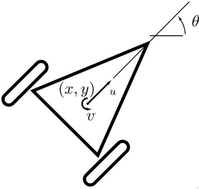
Figure 1: Unicycle robot kinematic
