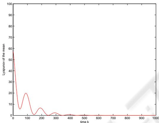
Figure 4: Lyapunov function of the mean of the multi-robot system in an obstacles-free environment.
