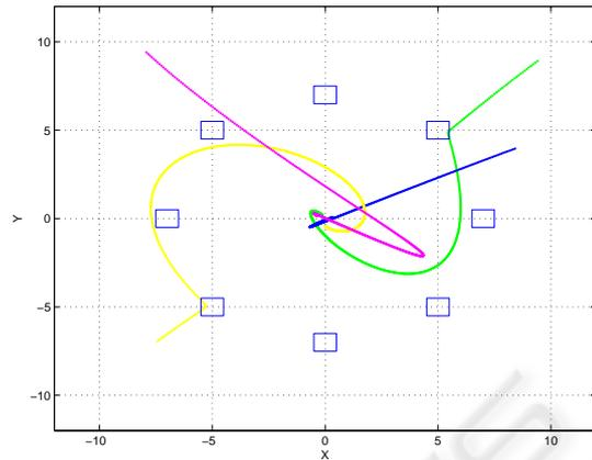
Figure 5: Motion of the individual robots in an environment with obstacles, considering a quadratic cost function.
