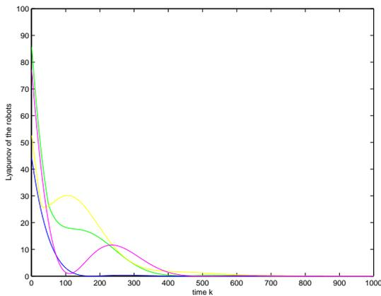
Figure 7: Lyapunov function of the individual robots in an environment with obstacles.
