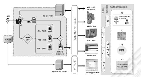
Figure 3: A PIC Deployment Scenario in a Healthcare Information System
